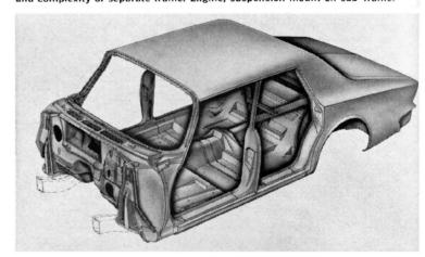
USE OF 4-DOOR roof panel on 2-door hardtops gives these more rear seat head and foot room, easier entrance. Seat height has been raised.
